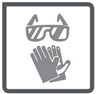
Gloves should be worn at all times when handling panels. Protective eye-wear should be worn when cutting panels.
